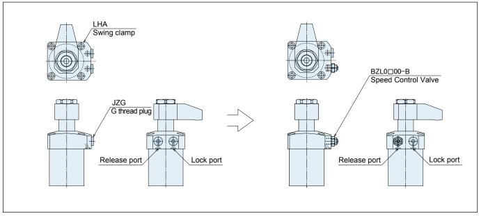
1. BZL (speed control valve), BZX (air venting valve) and JZG (G thread plug) can only be mounted on Piping Method C type.
